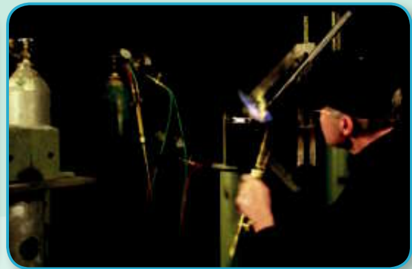
Oxygen and acetelene are used in welding metals
